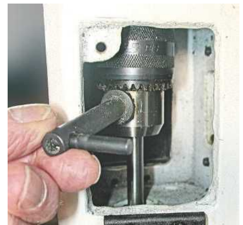
▲ Pic.4 He found that the chuck had to be very firmly tightened
